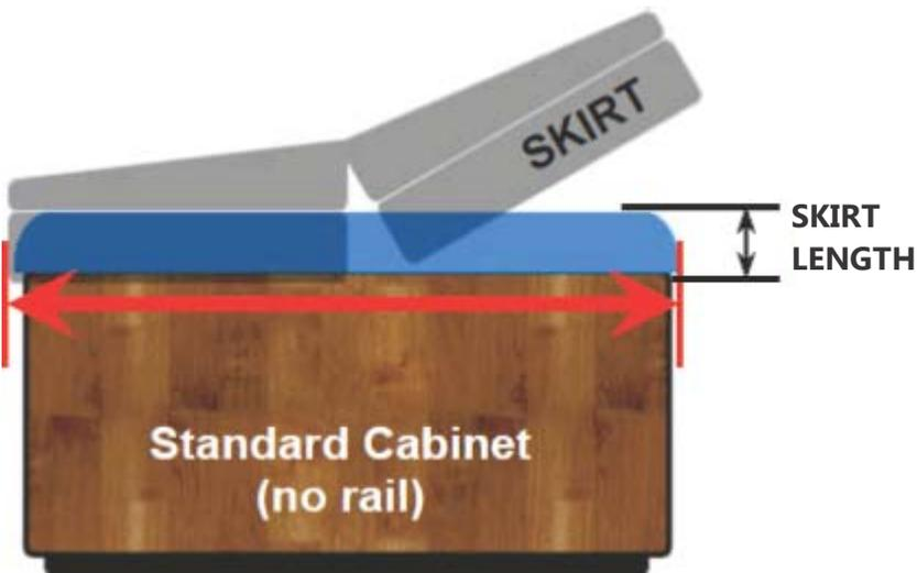
Most newer spas are made as shown here, with the acrylic shell lip overhanging the spa cabinet paneling. These spas are very easy to measure from the outside edge of the shell.
