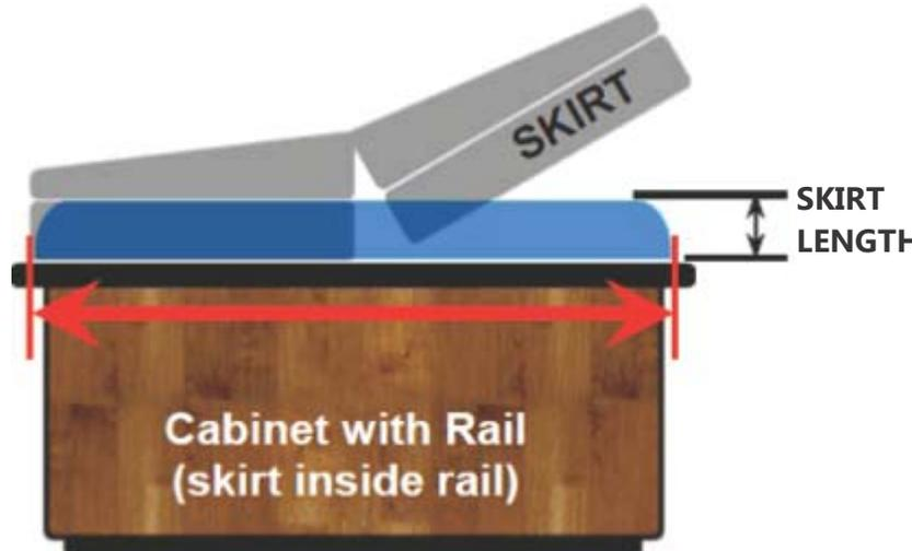
Shown here is the other way your cover can be made for spas which have an edge rail around the outside of the acrylic shell lip.
