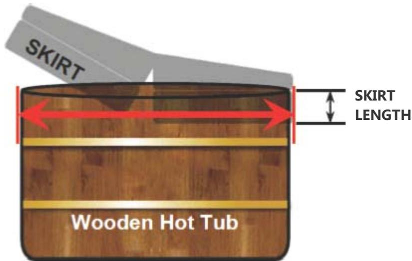
If you have a wood hot tub, be sure to measure the overall outside diameter of the tub (not the inside diameter of the opening).
