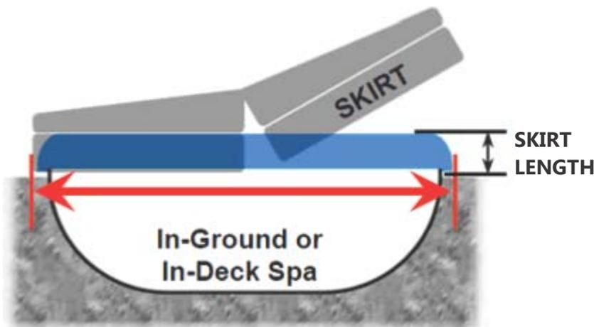
If your spa's acrylic shell rim is set directly onto a deck or concrete surface like this, be sure to measure the overall outside diameter of the tub (not the inside diameter of the opening). Make the skirt length a little shorter than distance from top of spa shell to the surface, so that it does not bunch up when the cover is closed.
